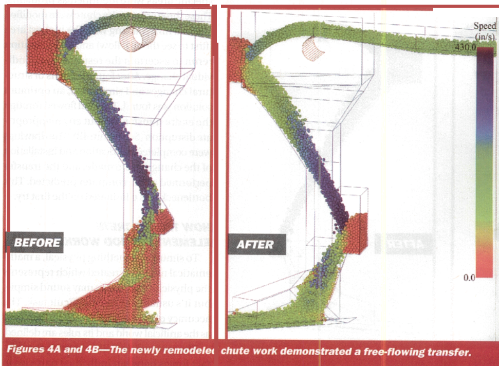
Figures 3A and 3B—The redesigned chute geometry allows material to flow more smoothly.
